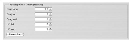
Longitudinal drag Drag coefficient (cd-value) in direction of flight
