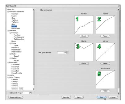
With this parameter you can set the pitch and throttle curves for the three flight phases "Normal", "Idle Up" (Acrobatic) and "Autorotation". Please note that the throttle curve is only used when the channel "Helicopter Engine" is set at "Automatic", otherwise the engine will be controlled by the throttle channel of your remote control (Compare paragraph 12.2).
