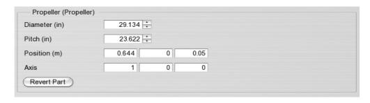
Diameter Propeller diameter in inches
