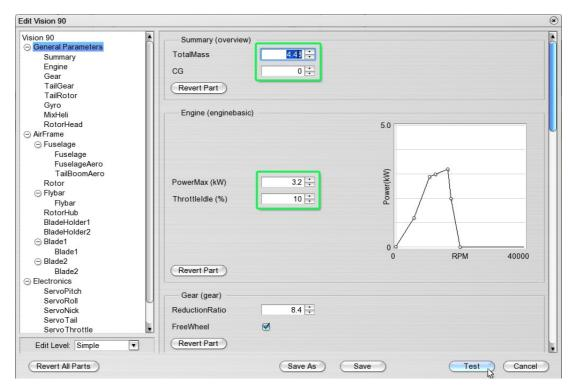
Select "General Parameters" and set the new values for the "Total Mass" and "Engine Power". Set the "Edit Level" at "Expert" and select the parameter "Rotor Head":
