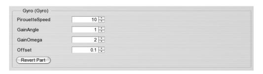
Pirouette Speed Pirouette speed. A value of 10 is equivalent to approx. 600°/ second.
