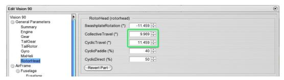
Here you can set all the entire control paths that are available for the collective and cyclical pitch. These are maximum values, that can be reduced by the pitch curve settings depending on the flight phases. Select "Mix Helicopter "in the parameter list:
