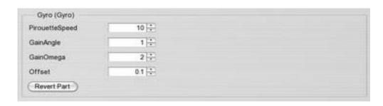
Pirouette Speed Pirouette speed. A value of 10 is equivalent to approx. 600°/ second.
