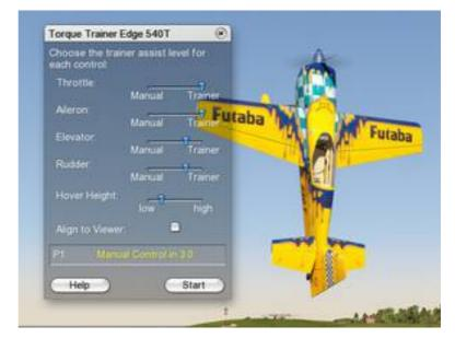
always attempt to position the model so that you can see it from above. If you want to allow rolling, move the slider for the 'Aileron' to 'manual'.
