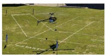
**Tip:** Improve the hover control of the model. Set in the advanced channel settings Expo from 0 to about 50 and downward adjust the overall channel range (rate) to about 60%. You may also fly with reduced speed by putting the engine on a channel manually.
