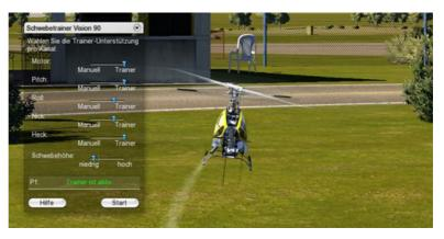
and learn to control the model, while the *Trainer* will help you with small corrections. If the *Trainer* has control over the tail rotor, it will try to align the model with the rear toward you.
