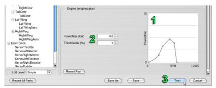
Before testing the settings, change the engine power: The power curve of the engine can be edited by shifting (1) the individual control points of the curve in the diagram using the mouse. Click a line between the control points and a new control point will appear automatically.
