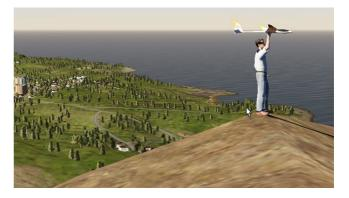
(windward side, to the right in the picture). (The glider could otherwise run out of energy on the leeward side). Gain altitude by flying with the updraft, turn and dive down on the leeward side and climb back up again to fly back below the boundary layer (on the leeward side of the ridge). Cross the boundary layer again from below close to the ridge, turn and dive down again on the leeward side, etc.
