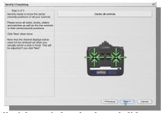
Identification of zero positions of all sticks, switches, knobs and sliders.
