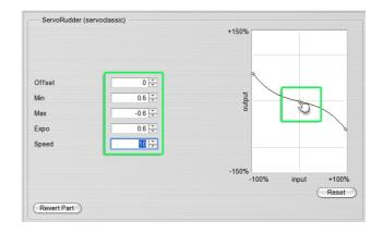
The control curve of the servo is displayed on the right side. For every stick position (*input*) the corresponding servo position (*output*) is displayed. Depending on the installation position of the servo, the curve either rises or falls until the correct control direction is reached as shown in the example.
