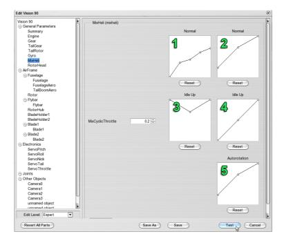
With this parameter you can set the pitch and throttle curves for the three flight phases *Normal*, *Idle Up* (*Acrobatic*) and *Autorotation*. Please note that the throttle curve is only used when the channel *Helicopter Engine* is set at *Automatic*, otherwise the engine will be controlled by the throttle channel of your remote control (Compare Paragraph 12.2).
