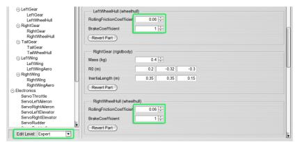
Select both *Left Wheel* and *Right Wheel* under *Aerodynamics* and set the rolling friction coefficient at 0.1 for each wheel.
