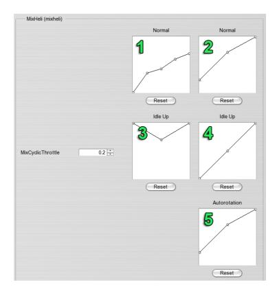
Throttle curve (1) Throttle curve for the flight phase Normal
