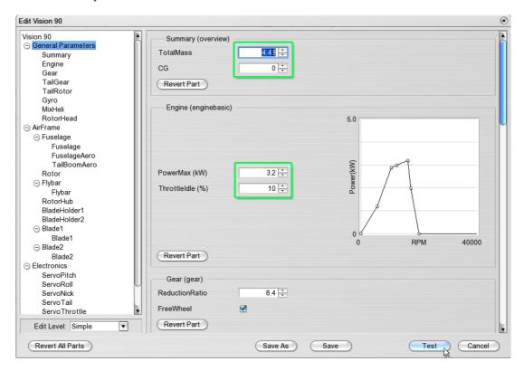
Select *General Parameters* and set the new values for the *Total Mass* and *Engine Power*. Set the *Edit Level* at *Expert* and select the parameter *Rotor Head*:
