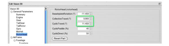
Here you can set all the entire control paths that are available for the collective and cyclical pitch. These are maximum values, that can be reduced by the pitch curve settings depending on the flight phases. Select *Mix Helicopter* in the parameter list:
