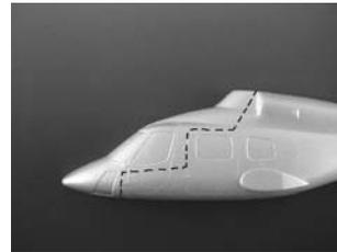
Separate fuselage and canopy along the marking using the scalpel. Particularly pay attention thereby to an even,
