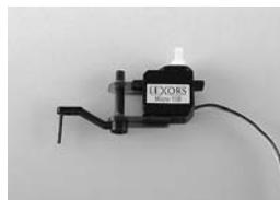
under the servo, and make sure that both bracket holes are aligned. Now push the axle into the brackets.
