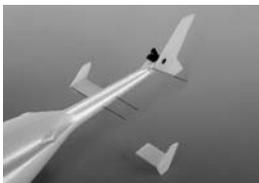
Glue one of the three thin carbon fiber struts with adhesive film to the vertical stabilizer fin as shown and glue the unit into place.
