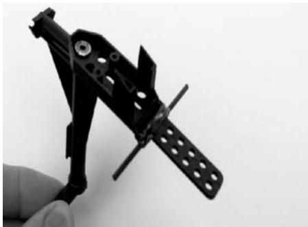
first unsolder the wires at the tail motor, and then pull them forward out of the tail tube.
