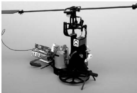
Assemble the Piccolo mechanics as described in the Piccolo instructions. Omit the skids, main motor, tail tube and tail skid.
