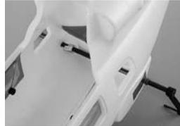
Continue sliding the axle through the right hole. Centre the axle and secure it with a second silicone ring. Now glue on the second landing gear leg.
