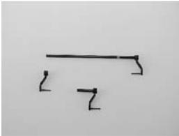
First drill out all wheel hubs to a diameter of 1.5 mm (1/16<sup>th</sup> in.) and CA glue the wheel half shells together. Now press one each of the 15 mm long wheel
