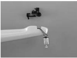
Modify the tail rotor housing as shown. Cut out the tail as shown and slide the tail motor wires into the opening created. Put the housing into the recess at the tail. Align the rear drive system to the vertical and longitudinal axis and glue it together with very little epoxy
