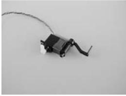
Put one of the axle brackets on the axle and insert the axle into the mounting bracket at the servo as shown. Glue the axle bracket under
