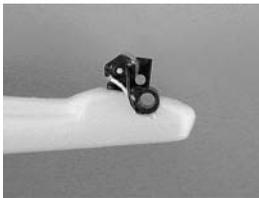
resin glue. Install the tail rotor gear box as described in the Piccolo Instructions, pages 18 and 19.
