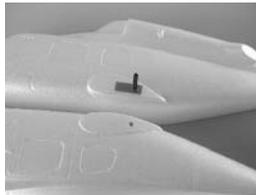
Cut out the vacuum molded mechanics support along the marked outline. Sand off the molded dome, until the shortened tail tube fits through the hole created. Do not sand off too much material, I to avoid any axle play. Using UHU Por glue the support as shown to the main former. Pay attention that the cut-out at the former is to the left, and also that the lower edge of the support runs parallel to the cut-out and the holes. Cut out for main shaft Axle
