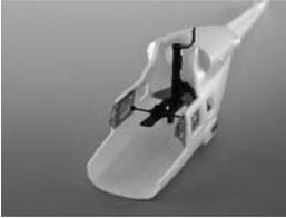
mechanics support, and that the mechanics mounts are flush with the fuselage seam. Mark the position of the mounts, take out the mechanics and glue on the mounts with UHU Por. Make sure that the fuselage fits snug over the mechanics.
