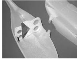
Using the scalpel cut out the openings for the carbon fiber main shaft on both fuselage half shells.
