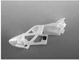
Cut out for roll servo pushrods -10 -10b / 10c- Cut out the recess for the nose wheel at the canopy. Glue the two polystyrene pieces into place as shown, as well as the two canopy locks. Put on the canopy and control the seat. If necessarily, work again on the fuselage, to give the roll servo linkage sufficient space for movement. When the canopy is on, make sure that the locks snap on to the mechanics holders.
