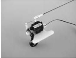
Widen the outer hole of the servo lever to a diameter of 1.5mm (1/16<sup>th</sup> in.) and put the lever perpendicular to the servo as shown.
