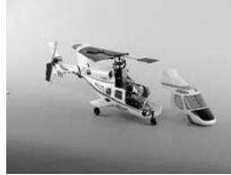
Now you can apply decals and ID numbers to the fuselage or paint the fuselage to your own desire. Paint with water soluble colors only, as they do not attack the material (for safety reasons try out on a piece of scrap material). An airbrush paint job is ideal, since it is laid on very thinly and thus is very light. When doing a lacquer finish you should definitely pay attention to the weight.
