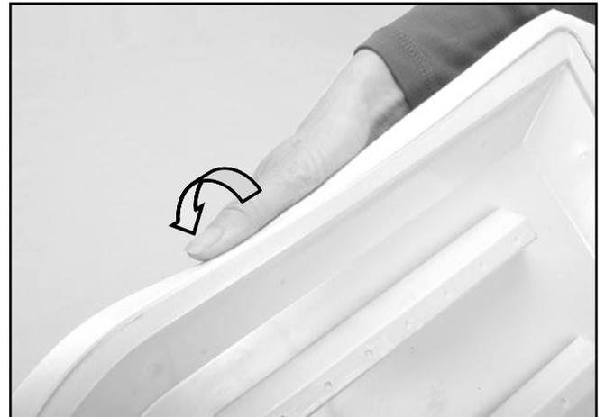
With a tapered drill cut the air release openings at the molded-in points by hand (alternatively you may also use a soldering iron). We do not recommend using a conventional drill as it would just rip the material apart.
