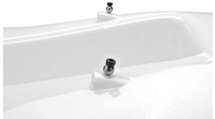
Then screw the two M2 threaded rods into the ball connectors and insert these into the CRP tubes. Slip a washer and a silicone sleeve (9 mm) over the exposed end and insert the rod into the oblong holes of the mount. Secure them on the opposite side with a self locking nut (do not tighten it yet). Now bend the threaded rod downward until the ball connector slips over the brass ball.
