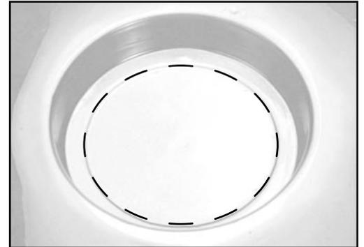
Cut on the inside along the edge with the razor blade knife before trimming the lower shell. As the lower shell is made of ABS plastic you may remove the excess material by simply bending it back and forth a few times.
