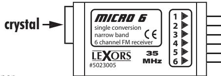
You may connect 6 servos to the receiver. If all connectors are occupied, the receiver power supply can be connected via a Y-cable.
