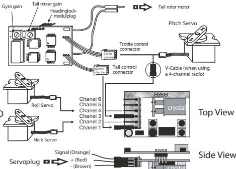
**Attention:** Carefully check that servo connectors and PRO board connectors correspond with the channel numbering system used by your transmitter before switching on.
