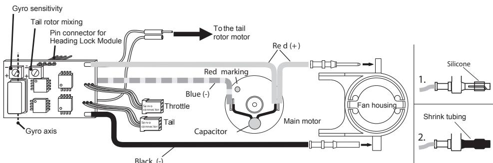
When mounting the PRO- board to helicopter please make sure the gyro axis runs parallel to the shaft of the main rotor.
