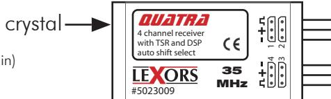
You may connect 4 servos to the receiver. If all connectors are occupied, the receiver power supply can be connected via a Y-cable. You also may use a Y-cable in case you want to use a 2 servo aileron set up.
